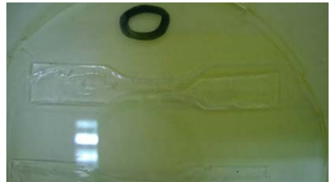
Figure 1.2: PU nano-composites with 0% DGO after exposure to UV radiation for 120 hours.
