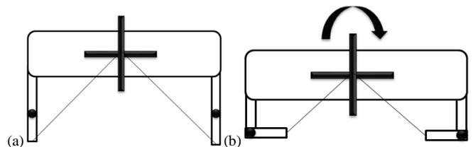
**Figure 9:** Folding Mechanism in (a) Standing Position & (b) Collapsed Position
