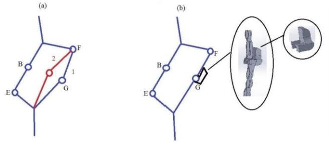
**Figure 6:** Bottom Triangle in (a) Jammed State & with (b) Anti-Jamming Mechanism
