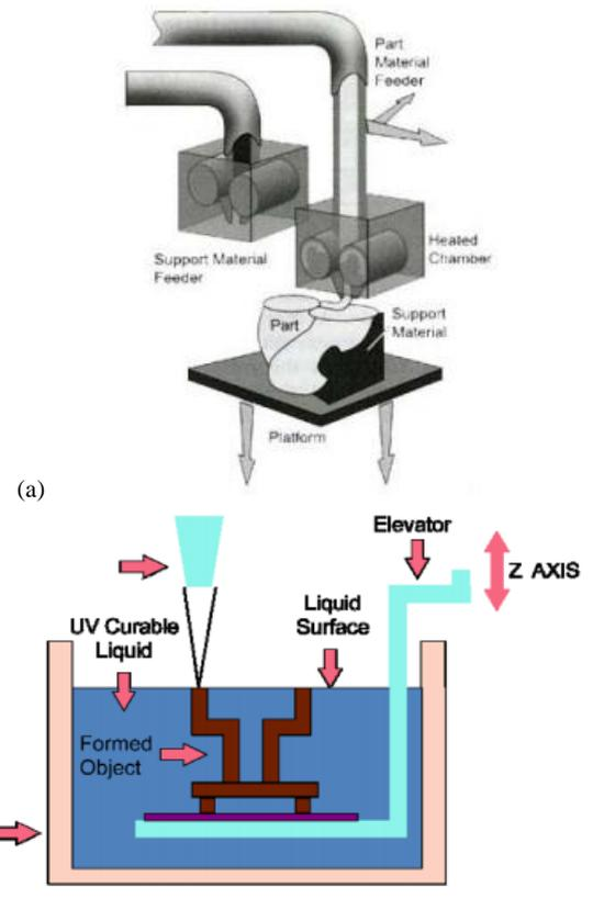
Figure 12: Schematic Diagram of (a) FDM Process; (b) SLA Process[5]
