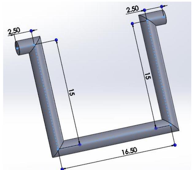
**Figure 18: Repeated Section of Crankshaft**
