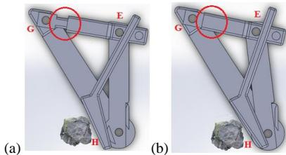
**Figure 8:** Spring System with (a) Spring Uncompressed & (b) Spring Compressed
