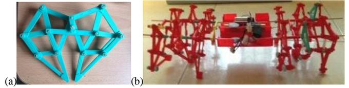
**Figure 3:** Preliminary Prototypes of (a) Pair of Legs & (b) 6-Legged Walking Model
