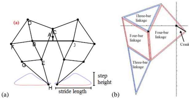
**Figure 2:** Jansen Linkage (a) Locus of 1 Pair of Legs and (b) Linkages in 1 Foot[3]
