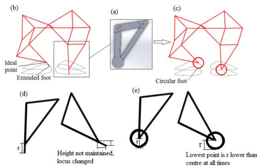
**Figure 4:** Effect of Circular Foot (a) Modified with Circular Foot, (b) Locus of Extended Foot, (c) Locus of Circular Foot, (d) Height not Maintained with Extended Foot & (e) Height Maintained at “ $r$ ” with Circular Foot
