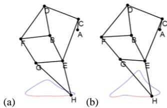
**Figure 7:** Step Height with (a) Original Length of GE & (b) Shortened Length of GE[3]
