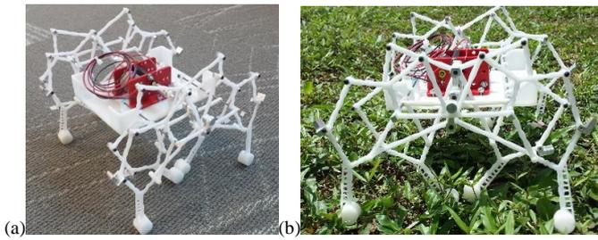
Figure 10: The Final 3D-Printed Model on (a) Carpet & (b) Grass
