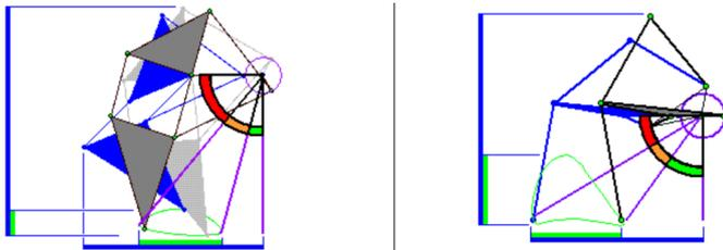
Figure 10: Jansen Linkage (left) & Klann Linkage (right) Comparison[8]
