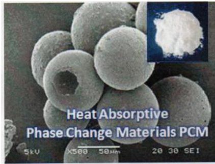
Fig 2: Scanning Electron Microscope image of encapsulated PCM
