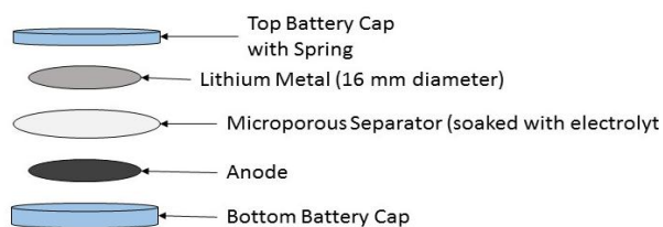
Figure 3: A diagram showing the assembly of a lithium ion battery
