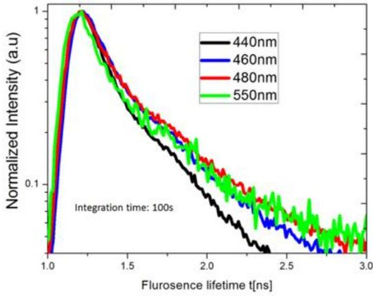
Figure 5 Fluorescence lifetime measurement by TRPL system for quantum dots incorporated quantum wells
