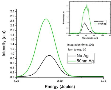
Figure 7 PL spectrum of the sample after depositing a layer of 50nm Ag. Inset gives the PL plot in nanometer
