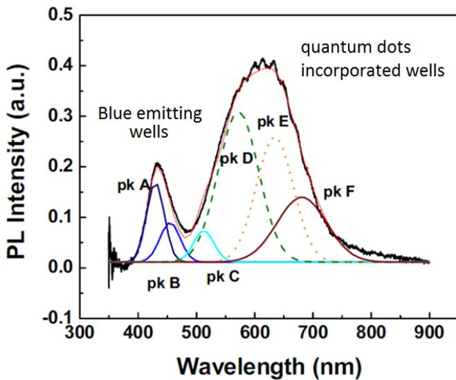
Figure 3 Photoluminescence scan for the quantum dots incorporated quantum wells with the fitted peaks as attributed by the different well layers
