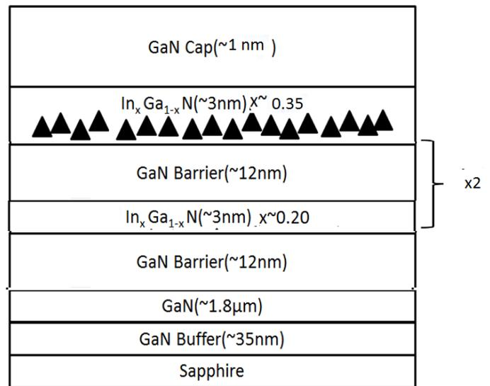
Figure 1 shows the schematic diagram of the growth MQWs structure with incorporated quantum dots
