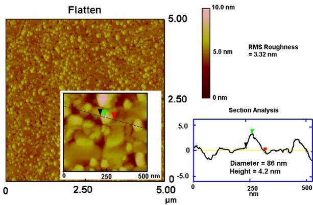
Figure 2 shows the AFM image of the quantum dots with a distribution of size from 30 nm-50nm for small quantum dots and 70 nm to 120 nm for bigger quantum dots distributed in the QWs structure. The inset shows a magnified image to determine the size of the dots.
