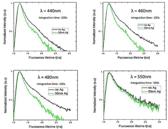
Figure 6 shows the TRPL (Normalized Intensity vs Fluorescence lifetime [ns]) spectra of the (50nm Ag) sample (in green performed) at different wavelengths at room temperature compared to the original sample (no Ag) plotted in black
