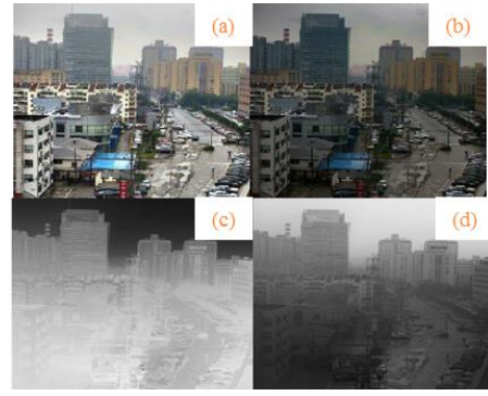
Figure 7. (a) guided filter output from section 3.2; (b) DCP output; (c) weight map for (a) in image fusion (section 3.3); (d) weight map for (b) in image fusion (session 3.3)
