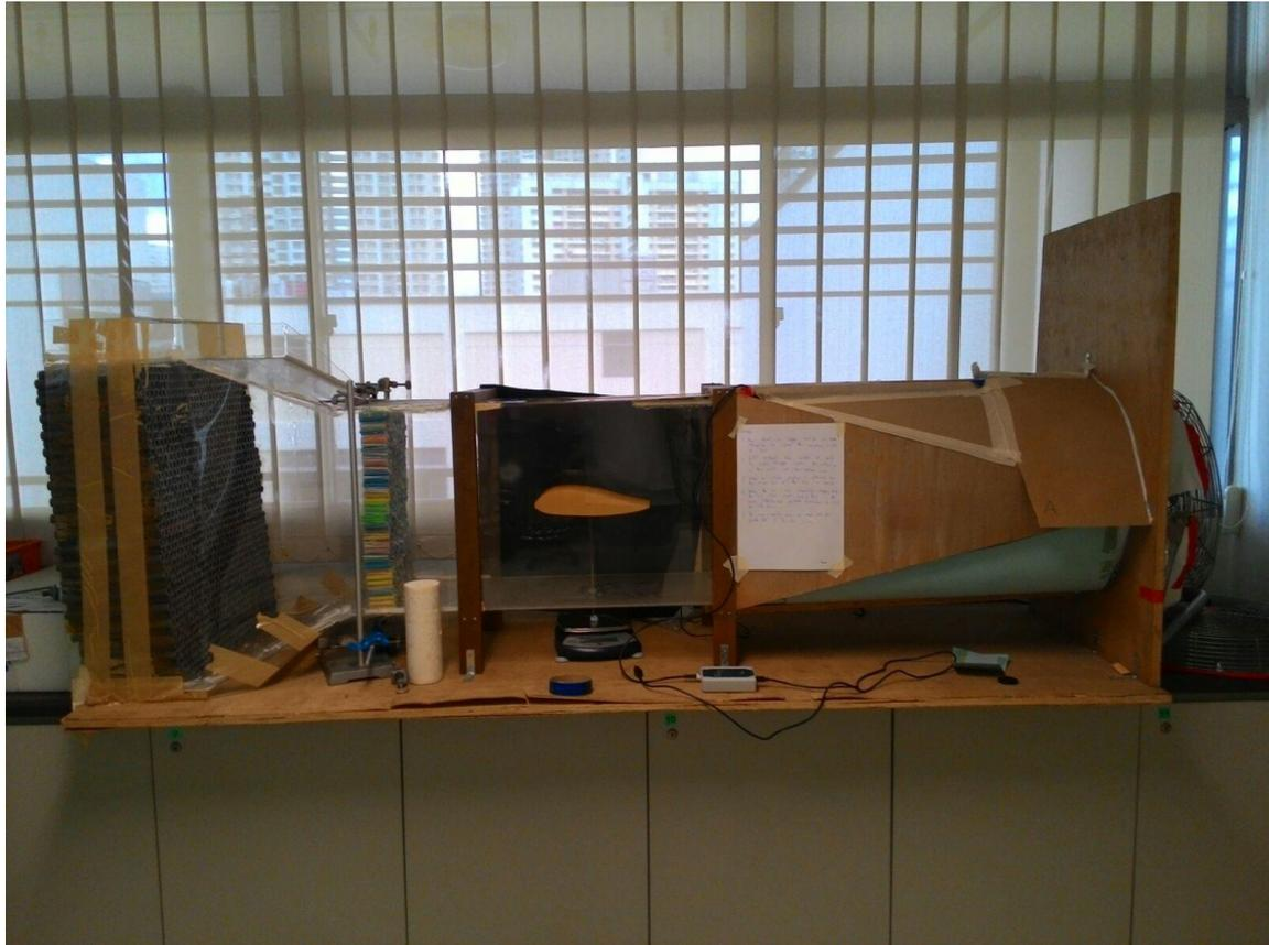
Figure 4.2: Wind Tunnel Set-up
