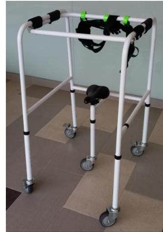
Figure 4. Walkie version 1.0 full-scale working prototype.
