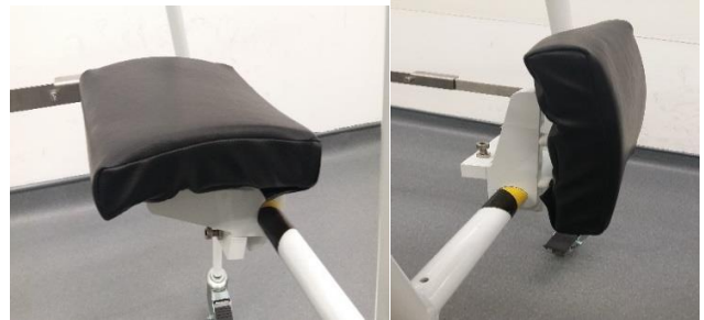
Figure 8. Retractable Seat pull down/up
